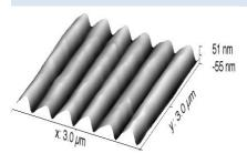
Left: 3D rendering of AFM traces of a grating pattern Below: A single unsmoothed AFM trace of a 1500 lines/mm grating with a blaze angle of  $1.1^\circ$
