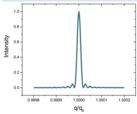
**Left:** Resolution function, R(q), reconstructed from the Fizeau data below, showing a resolving power of  $E/\Delta E = 50,400$
