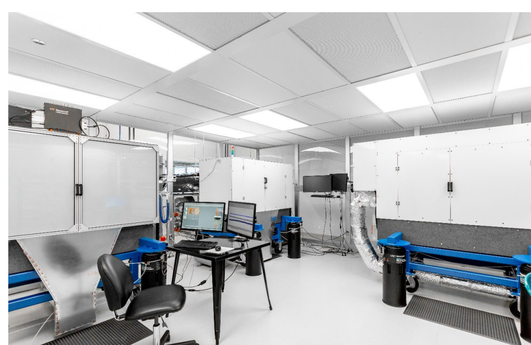
Figure 2. Inprentus manufacturing facility featuring three ruling engines in an environment-controlled cleanroom.
