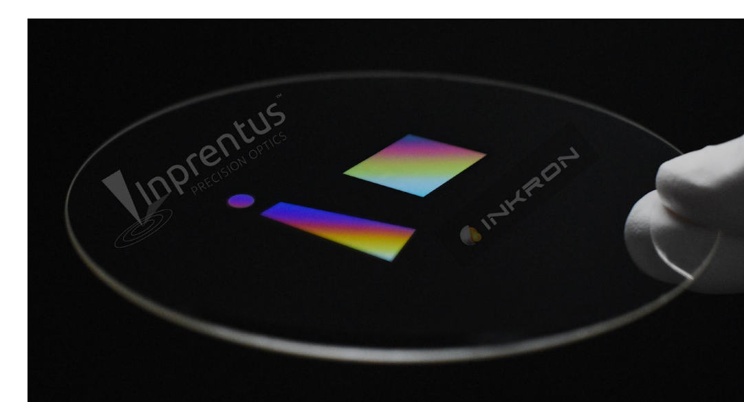
Figure 9. Three-grating AR waveguide in 1.9 index resin. Master fabrication by Inprentus and NIL replication by Inkron.
